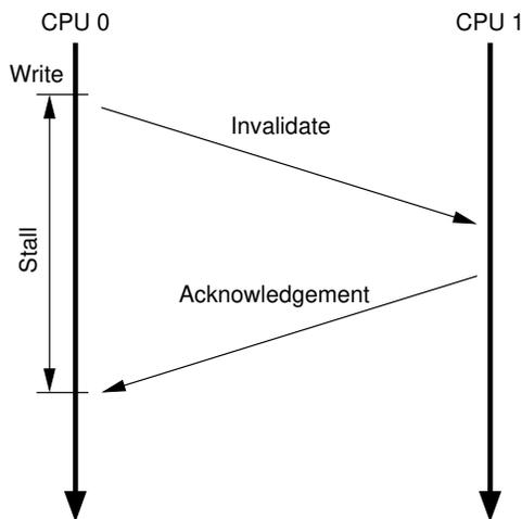
**Figure C.4:** Writes See Unnecessary Stalls
