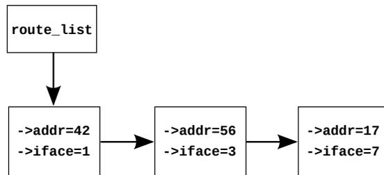
**Figure 9.1:** Pre-BSD Packet Routing List
