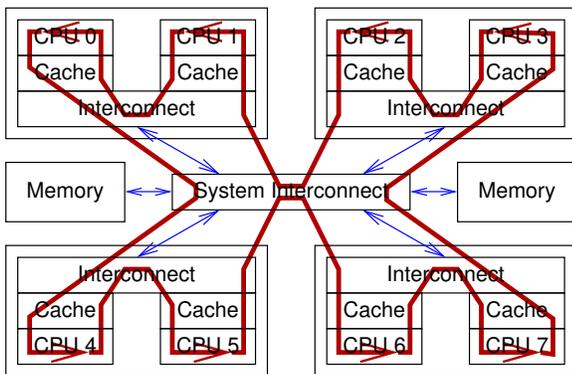
Figure 5.2: Data Flow For Global Atomic Increment
